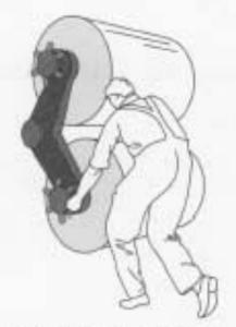
Blank newsprint rolls are inserted into the printing press in a process called web offset.
