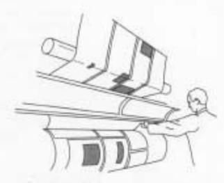
The plate cylinders press the image of the page anto a blanket cylinder, which in turn presses an image of the page anto the paper.
