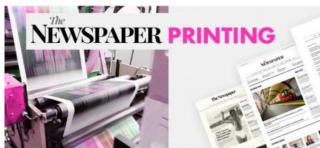
The plate cylinders then press the image of the page onto a blanket cylinder, leaving a version of the page's image on the cylinder's soft material. When the paper runs through the press, the blanket cylinder presses the image onto it.
