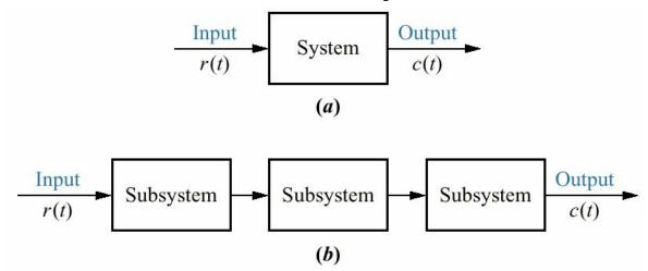
Note: The input, r(t), stands for reference input. The output, c(t), stands for controlled variable.
