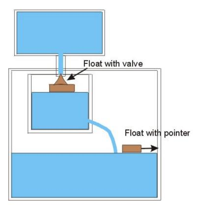
It kept time by regulating the water level in a vessel and, therefore, the water flow from that vessel.
