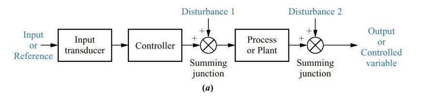
An open-loop system cannot compensate for any disturbances that add to the controller's driving signal or to the process output
