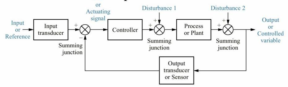
The closed-loop system can compensate for disturbances by measuring the output, comparing it to the desired output, and driving the difference
