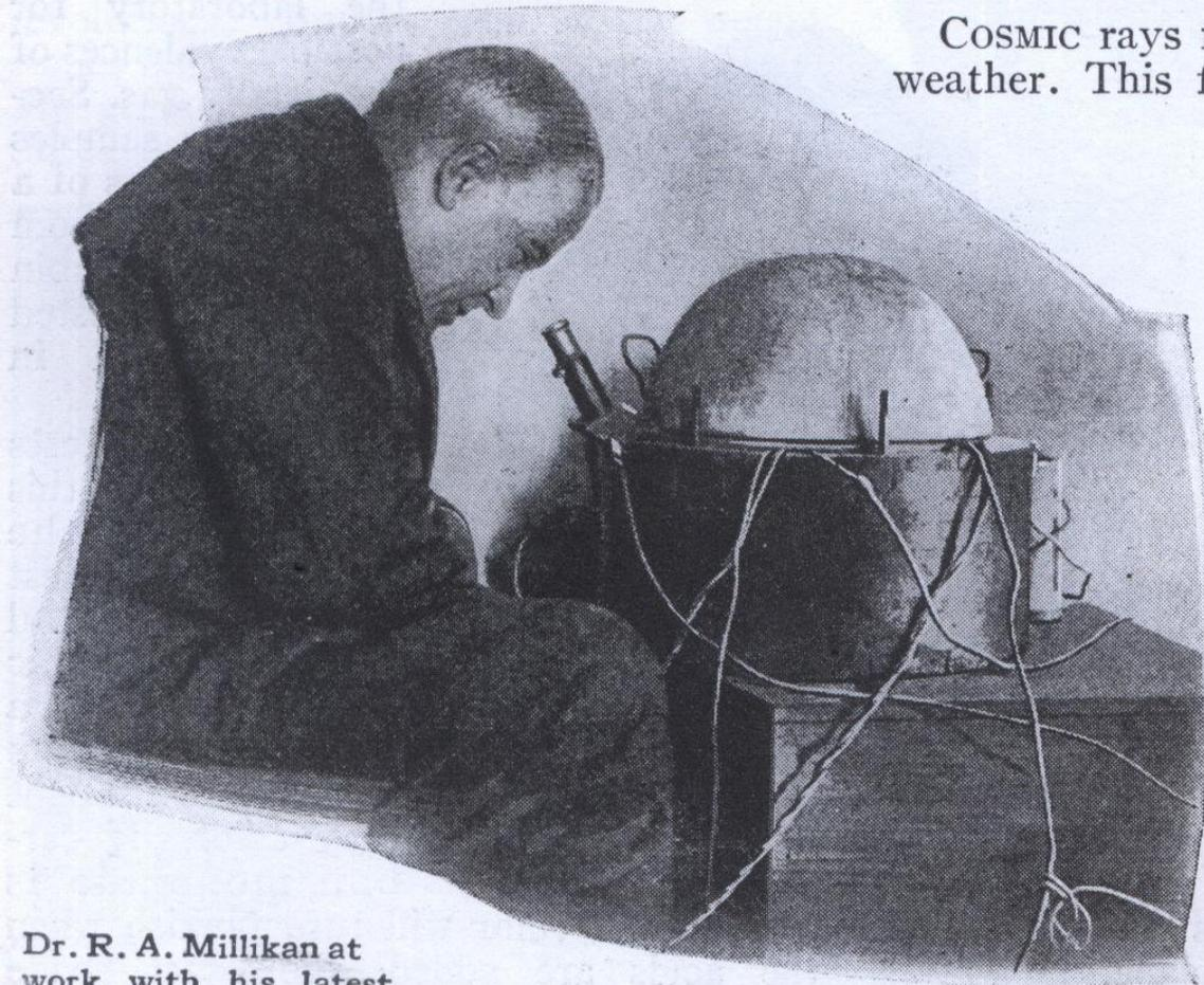
Dr. R. A. Millikan at work with his latest electroscopes, with which he is studying the cosmic rays. He believes these mysterious rays may be used in making reliable forecasts of the weather.
