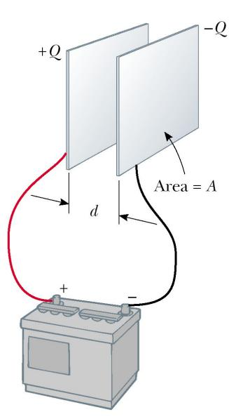
A parallel-plate capacitor consists of two parallel conducting plates, each of area A, separated by a distance d. When the capacitor is charged the plates carry equal amounts of charge. One plate carries positive charge, and the other carries negative charge.
