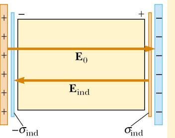
That's why dielectric's molecules produces induced electric field E<sub>ind</sub>, opposite to the external E<sub>0</sub>.
