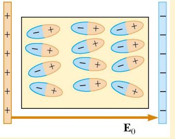
When an external field E<sub>0</sub> is applied, a torque is exerted on the dipoles, causing them to partially align with the field.
