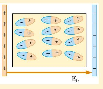
When an external Electric field is applied, its molecules partially align with the field. Now the dielectric is polarized.
