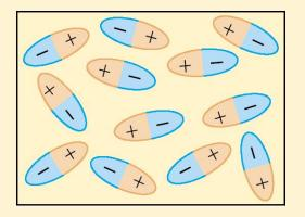
Dielectric can be made up of polar molecules. The dipoles are randomly oriented in the absence of an electric field.
