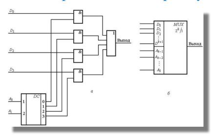
• Multiplexers are digital multi-position switches. They differ in the number of inputs and addressing methods. Multiplexers can select a specific channel and therefore they have other names-selectors or multiplexer selectors.
