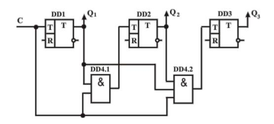
Counters are frequency dividers with different division coefficients. There are unidirectional and bidirectional ones. Divider counters are designed to divide the number or frequency of pulse repetition by a given division factor.
