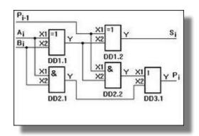
• An adder is a logical operating node that performs arithmetic addition of codes of two numbers. When adding arithmetic, other additional operations are performed: taking into account the signs of numbers, aligning the orders of summands, and so on.
