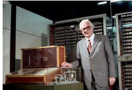
The Zuse Z1, built by Konrad Zuse in 1938 a binary electrically driven mechanical calculator with a 22-bit floating point value adder and subtractor, with some control logic making it capable of more complex operations such as multiplication and division.
