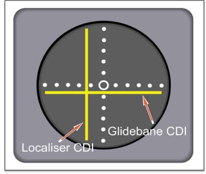
In <u>aviation</u>, the **instrument landing system** (**ILS**) is a <u>radio navigation</u> system that provides
