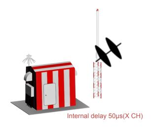
Distance =  $\frac{\text{Total travel time - }50\mu\text{s}}{12.36\mu\text{s/NM}}$
