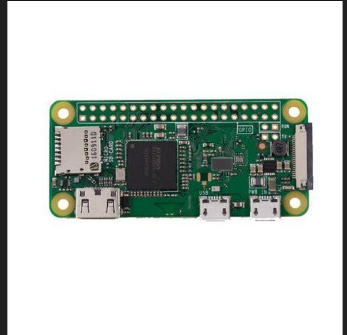
Raspberry Pi zero: 65mm x 30mm x 5mm
