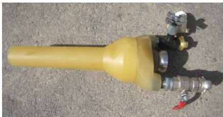
special spray gun V50 for shotcreting, max. 8mm grain size
