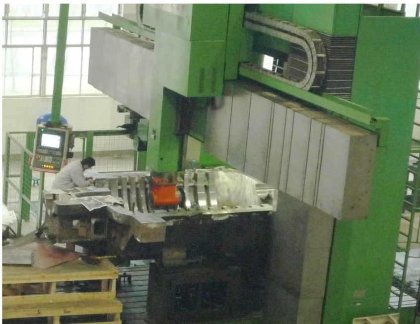
Machining of compressor casing at CNC Machining Center
