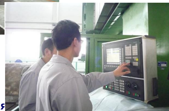
Beiyi Group CNC Double Column Boring and Milling Machining Center Length x width: 8m x 3m, table load is 80 tons)
