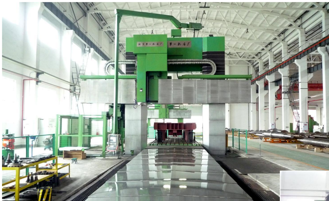
Beiyi Group CNC Double Column Boring and Milling Machining Center Length x width: 8m x 3m, table load is 80 tons)
