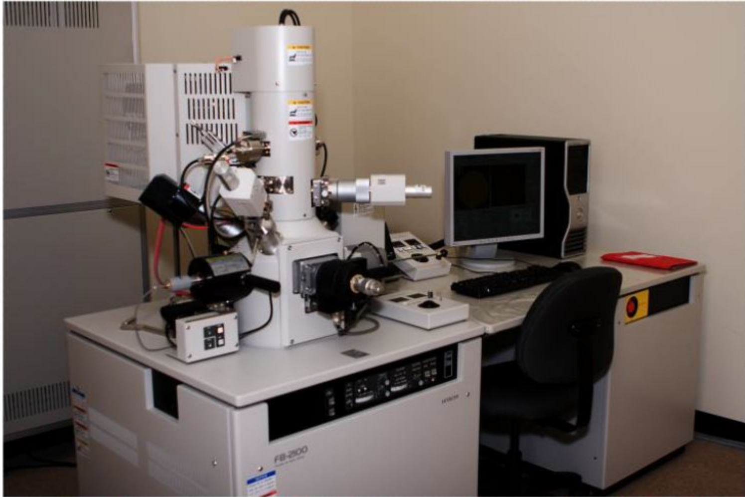
Focused Ion Beam System (FIB) Hitachi FB 2100
