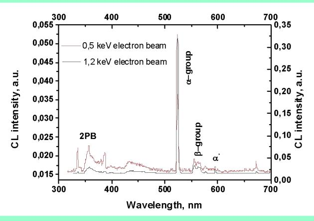
Luminescence spectra of solid N<sub>2</sub> excited with 0.5 keV and 1.2 keV electron beam
