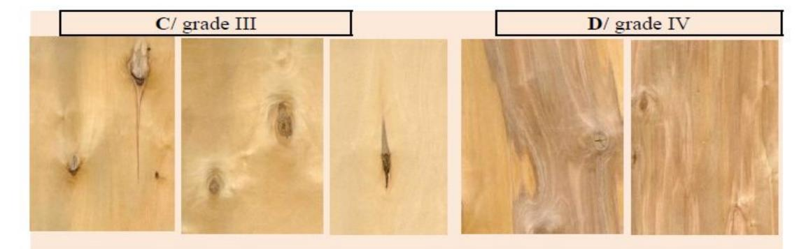
NOT ACCEPTABLE DEFECTS /ROUGHNESS / CRACKS (ALLOWED and LIMITED only to C and D grades)
