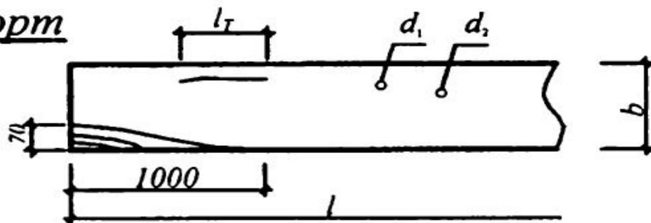
$$\begin{aligned} b < 100 & (d_1 + d_2) < \frac{1}{3}b & n=2 & l < \frac{1}{2}l \\ b > 100 & (d_1 + d_2) < \frac{1}{3}b & n=3 & \end{aligned}$$
