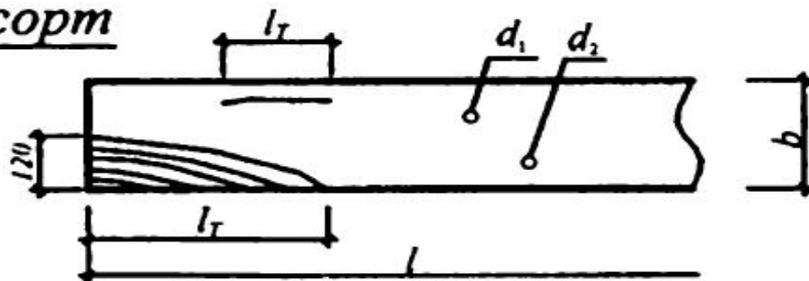
$$\begin{aligned} b < 100 & (d_1 + d_2) \leq \frac{1}{3}b & n=3 & l < \frac{1}{2}l \\ b > 100 & (d_1 + d_2) \leq \frac{1}{3}b & n=4 & \end{aligned}$$
