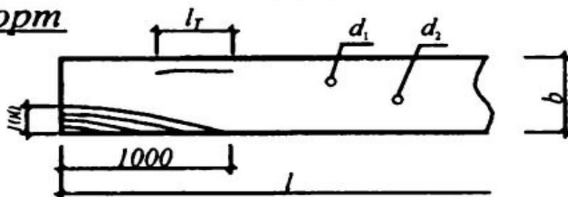
$$\begin{aligned} b < 100 & (d_1 + d_2) < \frac{1}{3}b & n=3 & l < \frac{1}{2}l \\ b > 100 & (d_1 + d_2) < \frac{1}{3}b & n=4 & \end{aligned}$$
