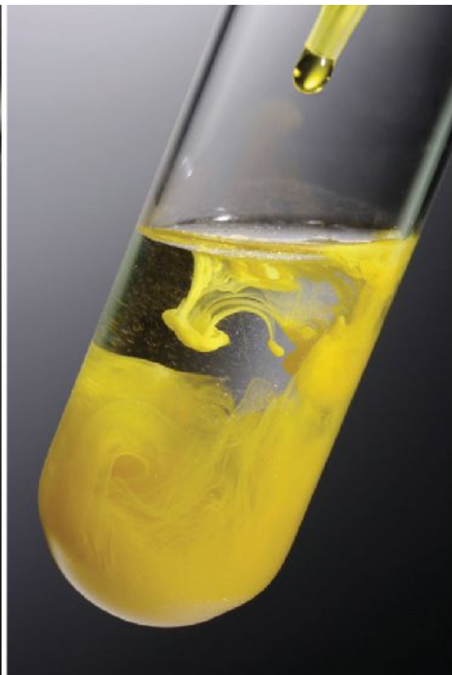
(b) Confirmation test for lead by addition of \text{Na}_2\text{CrO}_4(\text{aq}) : \text{PbCrO}_4(\text{s})
