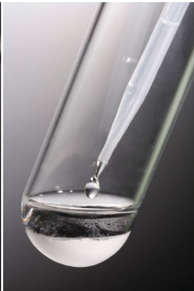
(c) Confirmation test for mercury by adding \text{NH}_3(\text{aq}) : \text{Hg}(\text{l}) + \text{Hg}(\text{NH}_2)\text{Cl}(\text{s})
