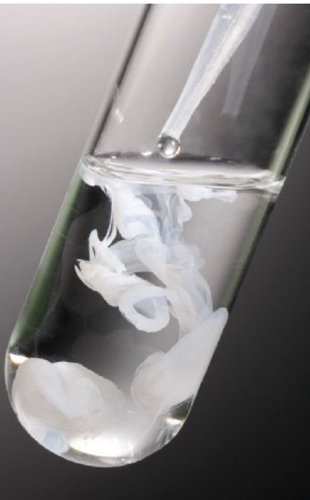
(a) Precipitation of group 1 cations by adding \text{HCl}(\text{aq}) : \text{AgCl}(\text{s}) + \text{Hg}_2\text{Cl}_2(\text{s}) + \text{PbCl}_2(\text{s})
