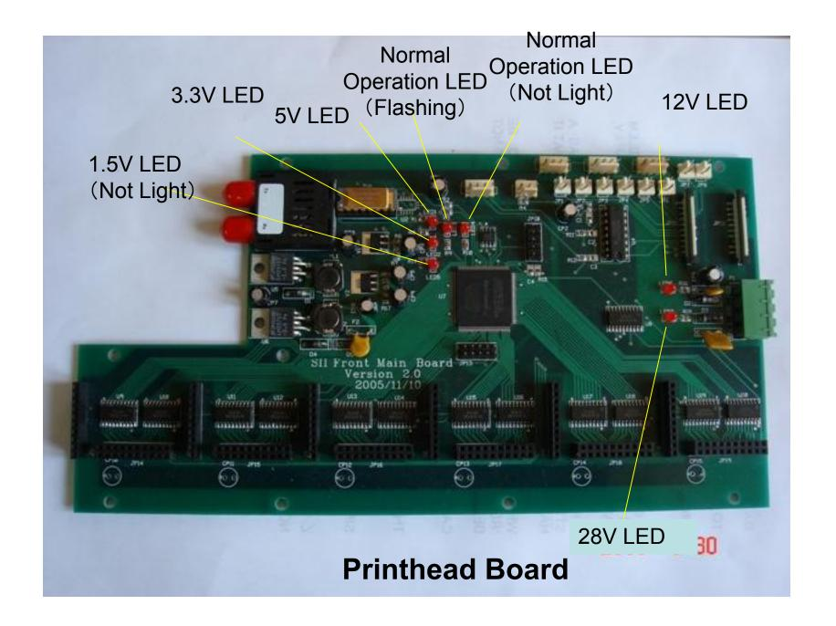
P.S.: When X and Y motor is working, corresponding LED will be on
