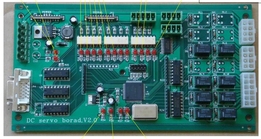
5V LED 3.3V LED Operation LED (Flashing)
