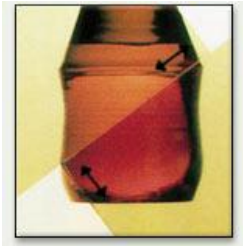
The purple-orange dichroism ( \text{Cr}^{3+} ligand-field colors) in a 3-cm-diameter synthetic ruby; the arrows indicate the electric vectors of the polarizers
