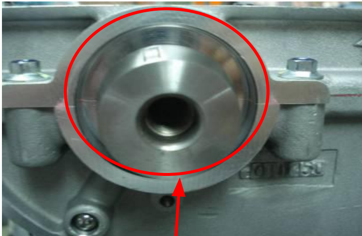
oil seal hole must be cleaned
