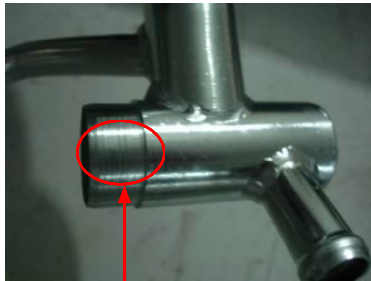
Pressing end of water outlet pipe
