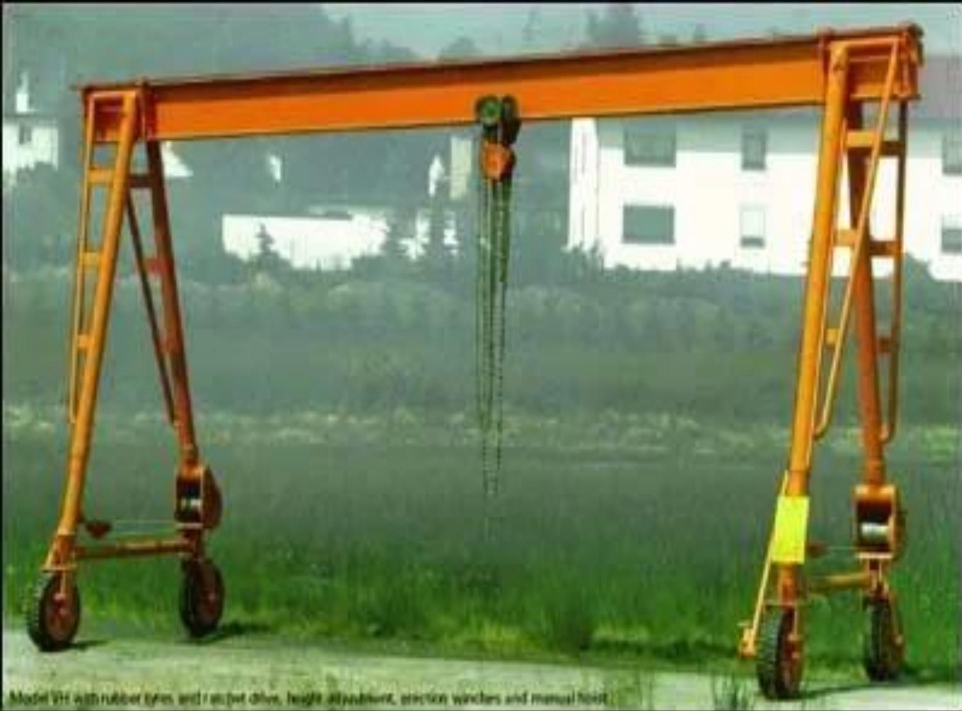
Model V8 with rubber tires and ratchet drive, height adjustment, electric winches and manual hoist.
