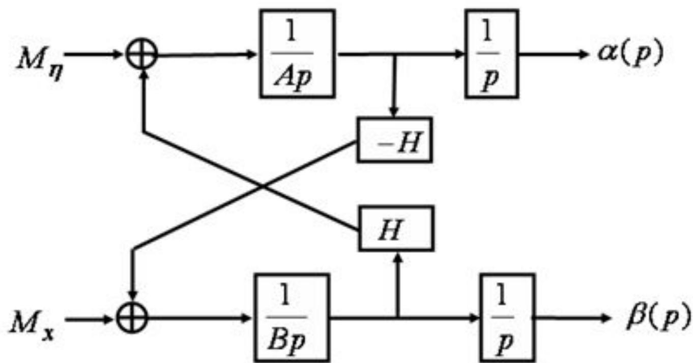
$$\begin{bmatrix} Ap^2 & -Hp \\ Hp & Bp^2 \end{bmatrix} \begin{bmatrix} \alpha(p) \\ \beta(p) \end{bmatrix} = \begin{bmatrix} M_\eta(p) \\ M_x(p) \end{bmatrix}$$
