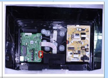
4. Remove the Power cables, LVDS cable, Function cable, LED cable.
