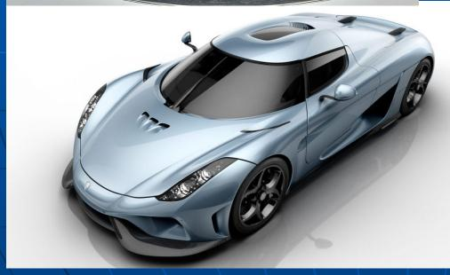
Koenigsegg Regera is first hybrid car of Koenigsegg and one of the most powerful hybrids in the world. Its petrol engine produces 1,100 horsepower, while 3 small electric motors add to its 1,500 HP total power. At a speed of less than 40 km / h, it can be driven only on electric motors.
