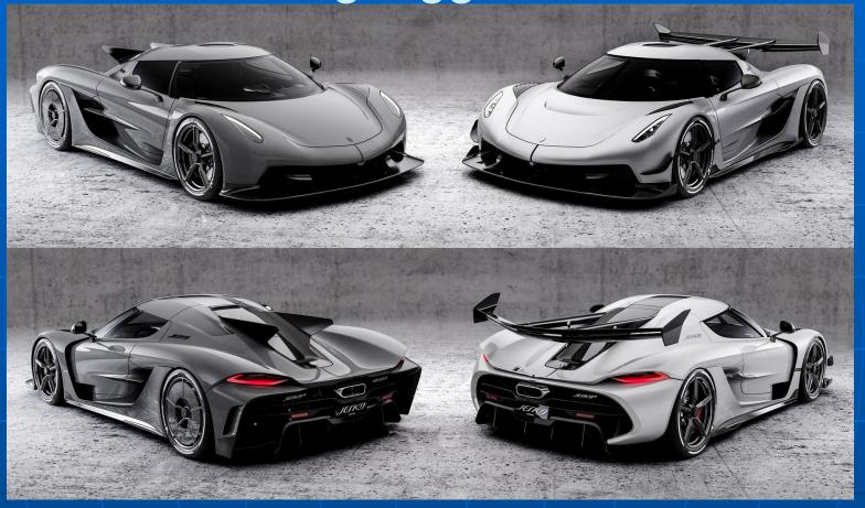
The Koenigsegg Jesko is not yet mass-produced, but the company expects it to be the fastest production car in the world. It is equipped with a 1600 horsepower engine and such aerodynamics that it must reach speeds up to 532 km / h, which will allow it to break the current speed record - the Bugatti Chiron was able to accelerate to 491 km / h last autumn.
