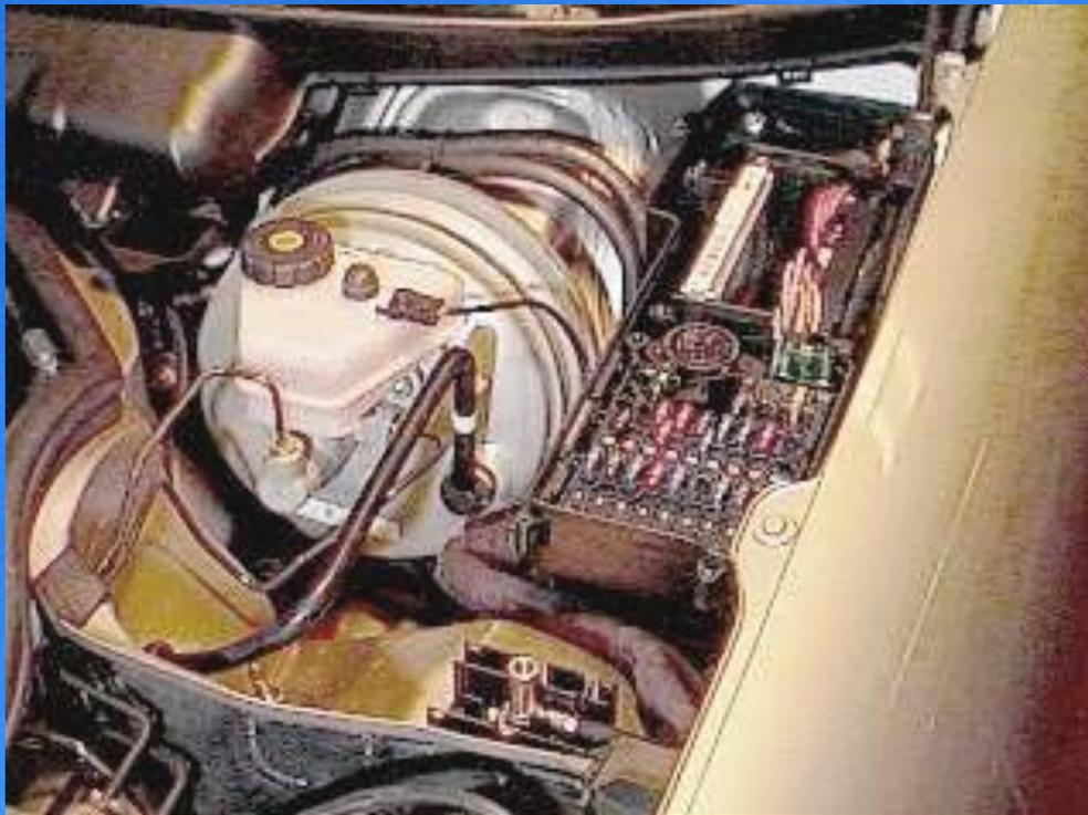
**In E-class (WDB210...) under the fuse box lid under the bonnet on the left**
