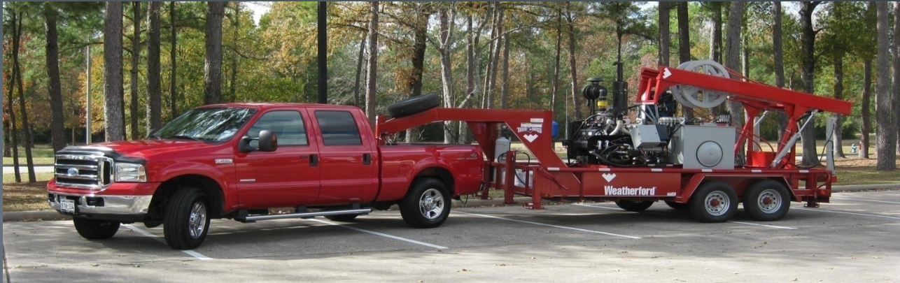
Portable Pumping Unit
