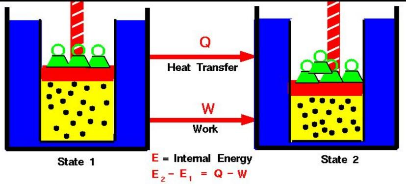
Any thermodynamic system in an equilibrium state possesses a state variable called the internal energy (E). Between any two equilibrium states, the change in internal energy is equal to the difference of the heat transfer into the system and work done by the system.
