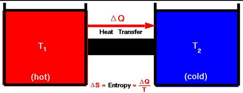
There exists a useful thermodynamic variable called entropy (S). A natural process that starts in one equilibrium state and ends in another will go in the direction that causes the entropy of the system plus the environment to increase for an irreversible process and to remain constant for a reversible process.
