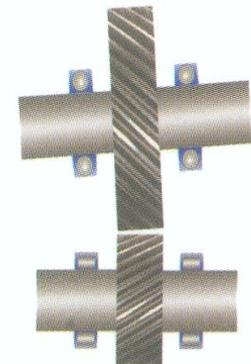
Gears mesh at an angle
