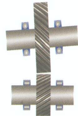
Gears mesh at an angle
