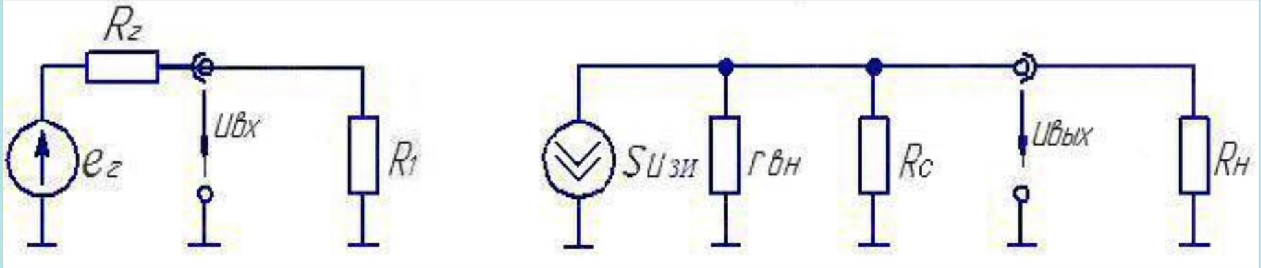
$$K_0 = \frac{u_{\text{вых}}}{u_{\text{вх}}} = -S(r_{\text{вн}} \parallel R_c) \approx SR_c$$
