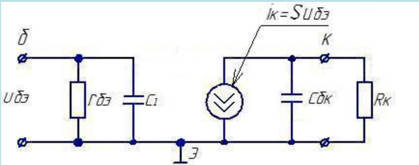
$$I_{mkб} = U_{mkэ} \omega C_{бк} (1 + 1/SR_к) \approx U_{mkэ} \omega C_{бк}$$
