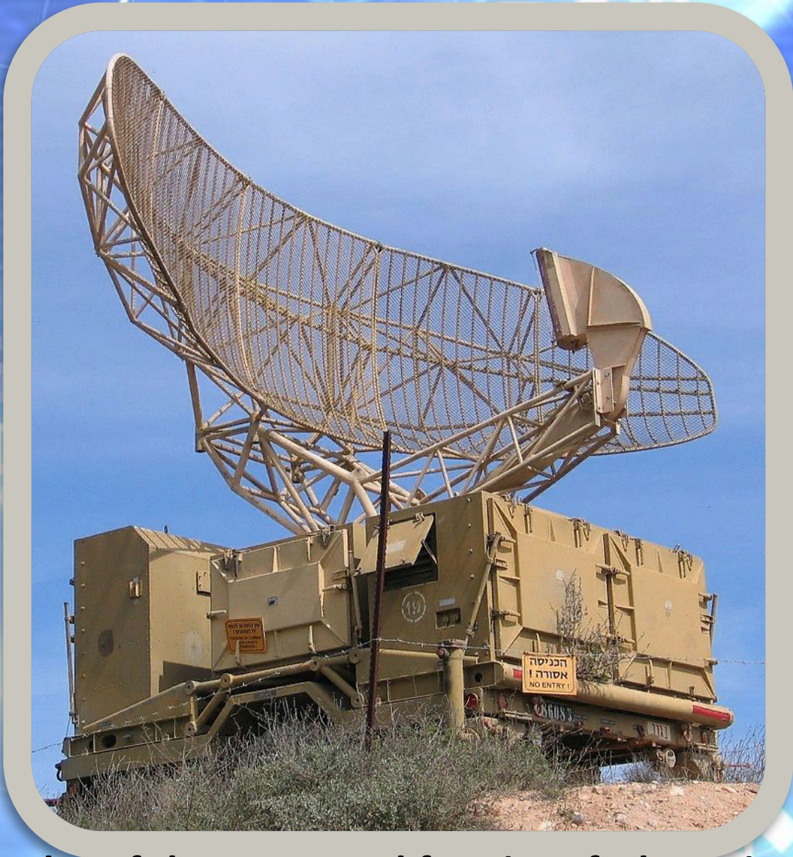
Radar of the type used for aircraft detection. It rotates steadily, skirting the air space with a narrow beam.
