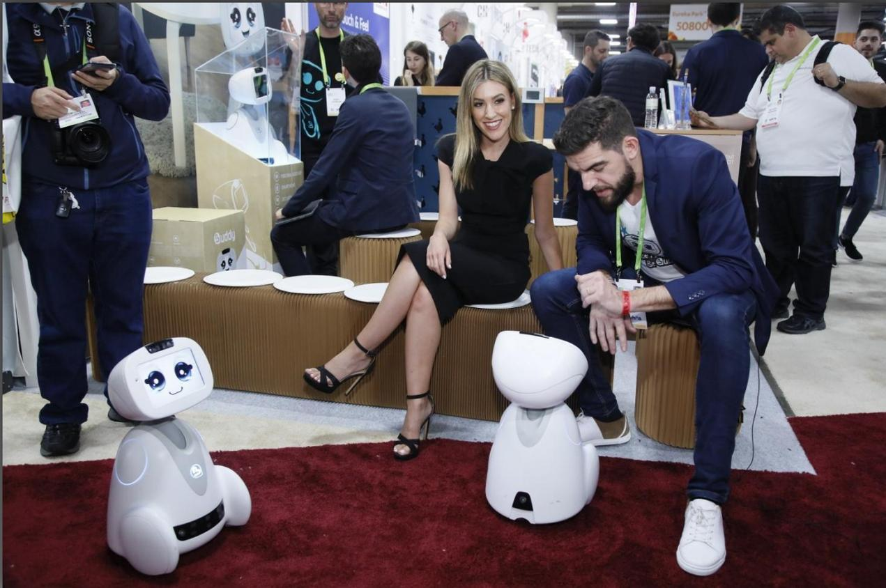
The fully mobile robot moves with two motorised wheels. With its sensors, cameras, and microphones, the robot is able to hear and speak. The robot can help the family with daily tasks, protect the home, entertain the children, and interact with other smart connected devices in the home
