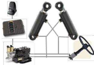
Joystick steering Parallel with steering Orbitrol
