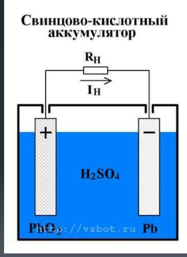
Accumulation of electricity: lead-acid batteries
