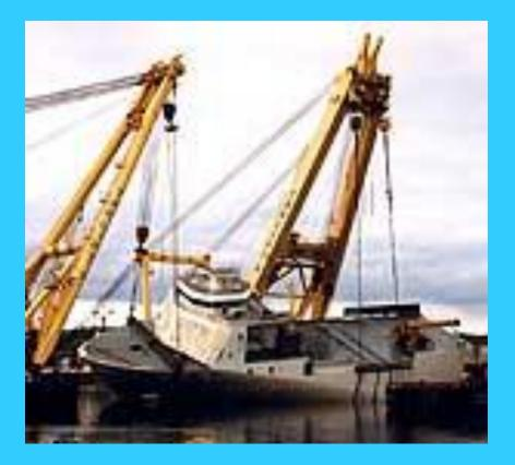
A salvage vessel has been equipped with heavy derricks to lift wrecks from the seabed.
