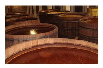
Once fermentation is complete, the mosto may be left to settle for about 12 hours to richen. The fermentation yields a liquid with about 5-7% alcohol. This product is then normally double-distilled in traditional copper pot stills (called alambiques) or by use of modern stainless-steel column stills to increase its alcohol percentage and separate the desired volatile substances from the undesired ones.
