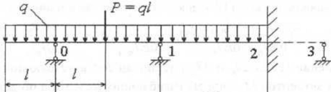
$$l_n M_{n-1} + 2(l_n + l_{n+1})M_n + l_{n+1}M_{n+1} = -6 \left( \Omega_n \frac{a_n}{l_n} + \Omega_{n+1} \frac{b_{n+1}}{l_{n+1}} \right)$$
