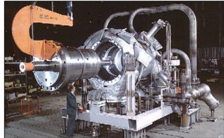
SST-700 (ST6): dual casing turbines
