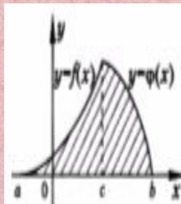
$$S = \int_a^c f(x) dx + \int_c^b \varphi(x) dx$$
