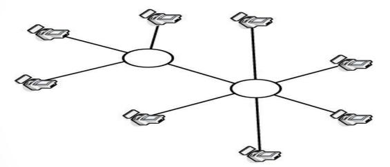
True star topology configurations are rarely seen in LAN implementations. However, the point-to-point connections made between hosts and switches look like a star topology. A star hub differs from an Ethernet switch or hub by how traffic is managed at the central connection.
