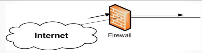
That way you can limit traffic to certain types of communication, block access of potentially hazardous applications, and even place restrictions on source and destination address information.
