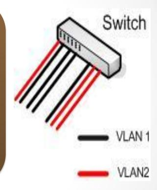
VLANs have become a popular segmentation option for LANs. Routers are still the primary means of segmenting over a wider area and between wide area links.
