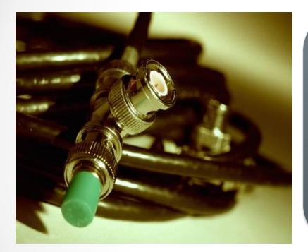
10Base2 had devices connecting directly to the cable in a branching or daisy-chain configuration. Connections were made using a BNC connector. Both types of cable had to be terminated at each end with a 50-ohm terminator to ensure signal quality.
