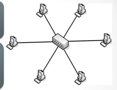
When a switch is used, it compensates for one of the weaknesses of the bus topology. The switch adds traffic control by buffering transmissions at the port, thereby avoiding most collisions. The switch ports can be configured so that they act as a single cable segment for addressing purposes.
