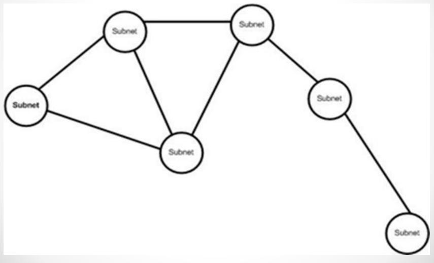
With VLANs, switches are used to segment the network, and segmentation is usually by port. A VLAN can be made up of ports assigned from a single switch or made up of ports gathered from multiple switches. Each VLAN will have a different ID number and a different assigned IP address. A VLAN can be associated with multiple subnets.
