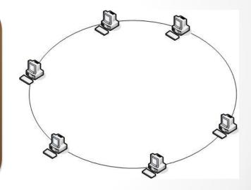
Some ring topologies use a double ring, that is, two rings that send signals in opposite directions. This enables the ring to compensate for a break or a failing node until the problem can be repaired.
