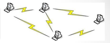
In ad-hoc mode, you configure wireless devices to communicate directly with each other. This enables the devices to share files and other resources with each other, but not with any wired network devices.
