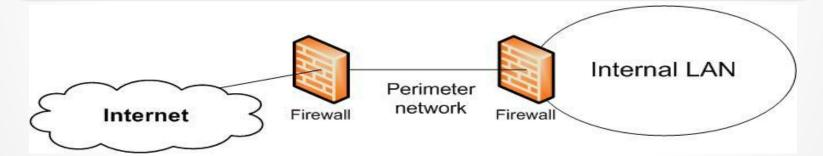
The primary purpose of a perimeter network is that it gives you a place to deploy devices that you want to share with the world at large.
