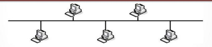
In a bus topology, all nodes receive every transmission at effectively the same time. If a transmission is not addressed to a specific node (or addressed as a broadcast), the node will ignore the transmission. This type of bus topology is sometimes called a linear bus.
