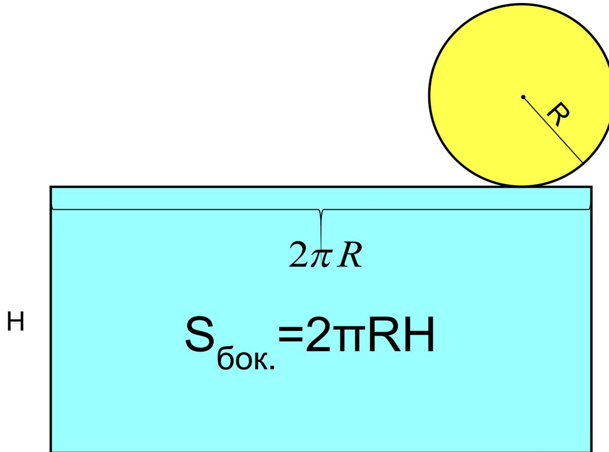
$$S_{\text{полн.}} = 2S_{\text{осн.}} + S_{\text{бок.}} = 2\pi R^2 + 2\pi RH$$
