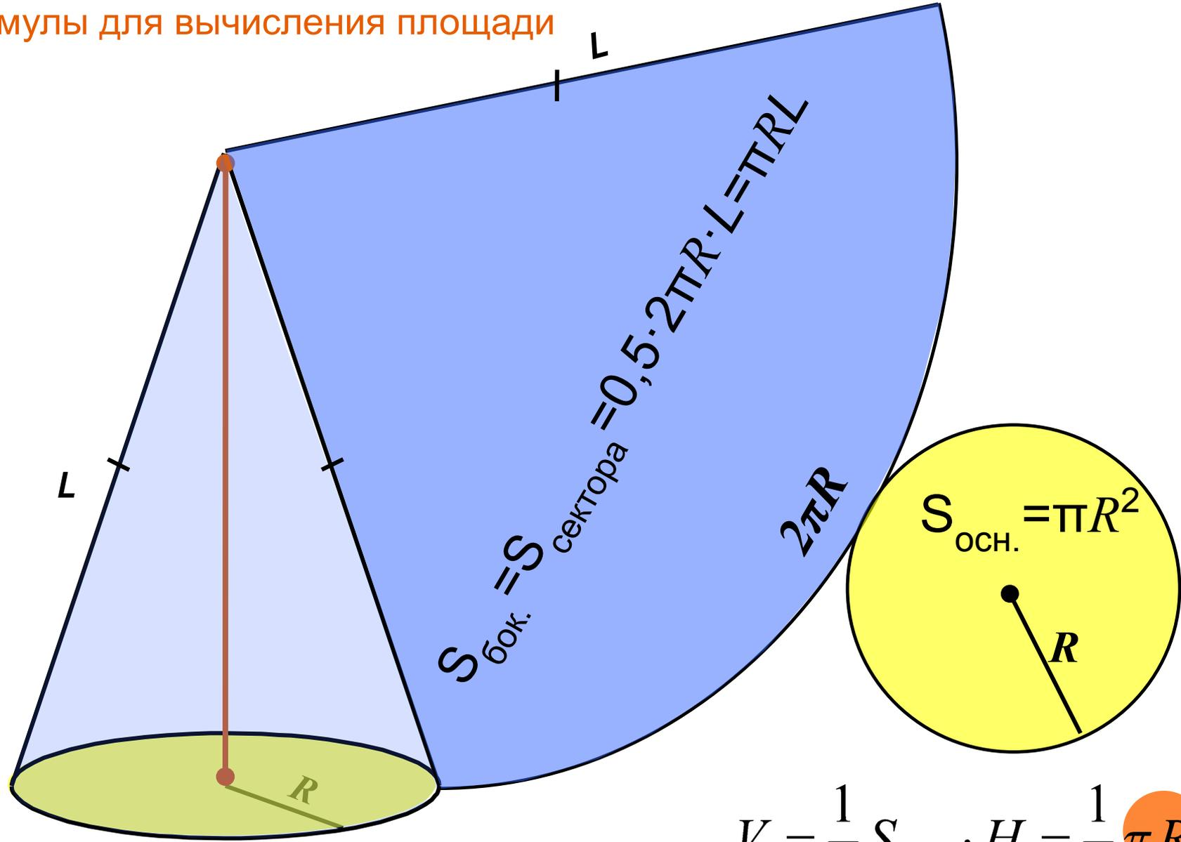
$$S_{\text{пов.}} = S_{\text{бок.}} + S_{\text{осн.}} = \pi R L + \pi R^2 = \pi R(L + R)$$
