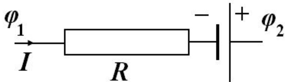
Diagram of a circuit segment showing a resistor  $R$  with voltage drop  $\varphi_1 - \varphi_2$ . The current  $I$  flows through the resistor from point 1 to point 2.
