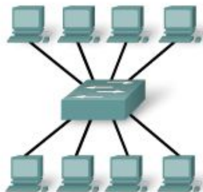
One large, central switch
