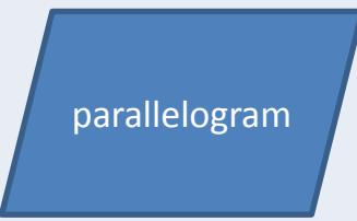
parallelogram | Data.     | This shape indicates that data is entering or leaving the process. It is sometimes referred to as the Input/Output pattern.                                                   |
