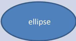
ellipse         | Start/End | This shape should be used to represent the first and last steps of the process.                                                                                               |
