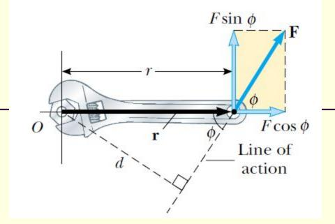
The force F has a greater rotating tendency about axis O as F increases and as the moment arm d increases. The component F  $\sin \varphi$  tends to rotate the wrench about axis O.
