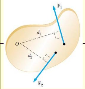
The force  $F_1$  tends to rotate the object counterclockwise about O, and  $F_2$  tends to rotate it clockwise.
