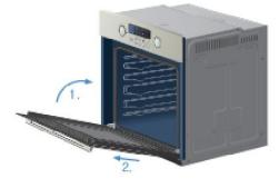
Close the door by approximately 45°. With both hands, grasp the sides of the oven door at its middle and pull-lift until the hinges can be taken out.
