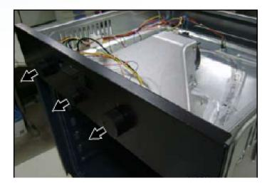
6 - 4 - 3 Remove two screws at both sides of assy control box, lift up assy control box and pull forward to separate.
