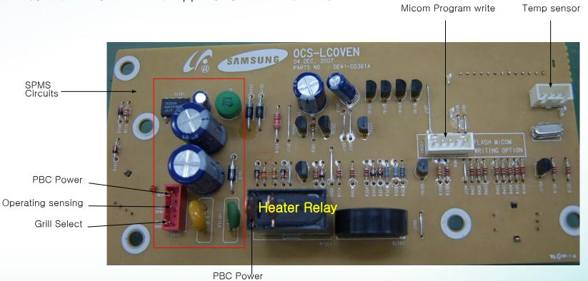
Please cut off the Main Power during dissamblling PCB or checking the part of PCB. Because there is no Insultion-Trans bewteen Main-Power and 2<sup>d</sup> Low-Voltage
