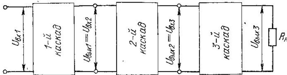
$$K_u = K_1 K_2 K_3 \dots K_n \quad K_u = U_{\text{ВЫХ3}} / U_{\text{ВХ1}}$$
