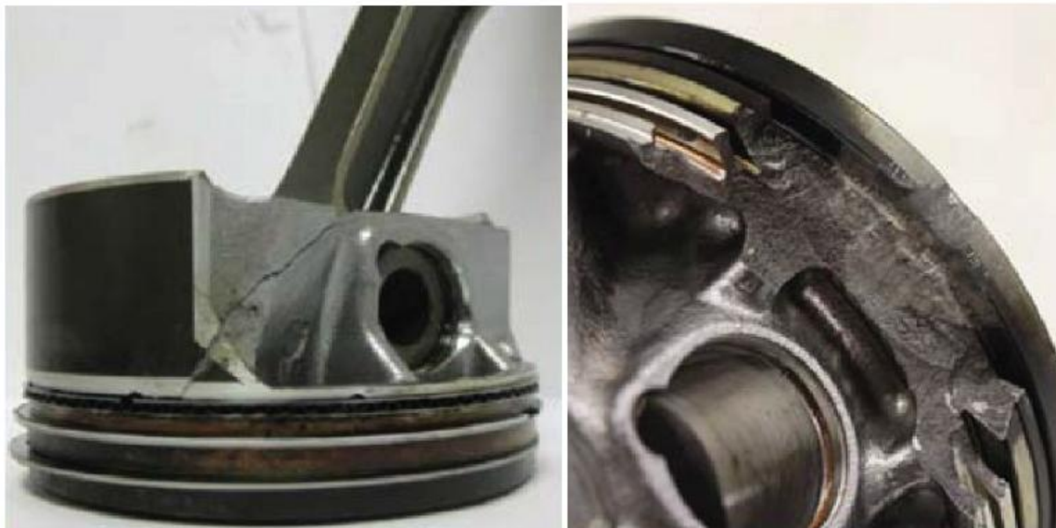
Two examples of piston damage due to LSPI observed during testing at Southwest Research Institute ®
