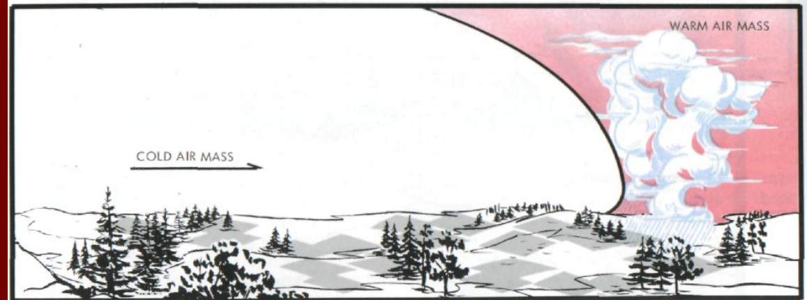
Top.—Lifting of warm, moist air, as it is forced up the slope of a warm front, produces widespread cloudiness and precipitation.
