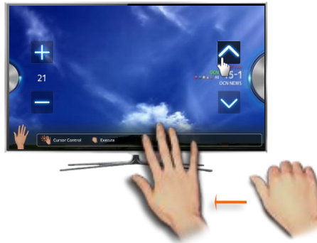
4. Grabbing hand is a Click. (If you maintain hand grabbed, TV execute channel up consecutively)
