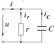
$$\overline{I} = \overline{I}_{r} + \overline{I}_{C}$$
