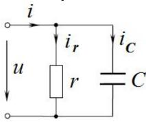
$$\overline{I} = \overline{I}_{r} + \overline{I}_{C}$$
