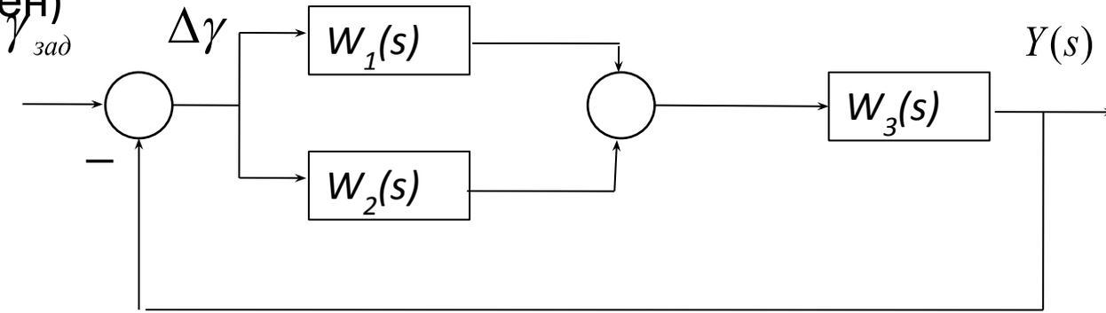
$$W_1(s) = k_1 \quad W_2(s) = k_2 s \quad W_3(s) = \frac{k_3}{s(T_3^2 s^2 + 2T_3 \xi s + 1)}$$
