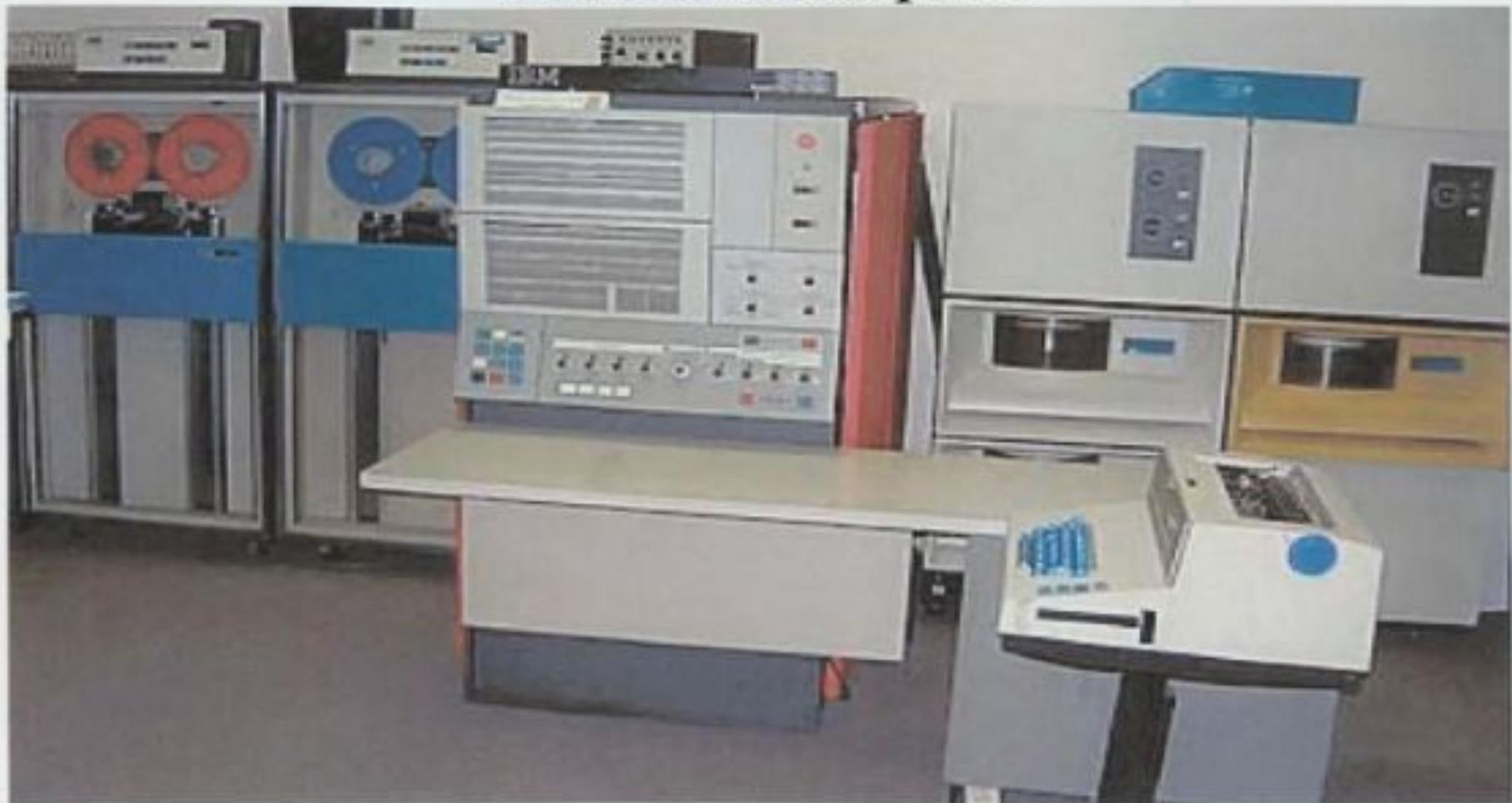
IBM System 360, Model 30, Memory size: up to 64K bytes, 1965
